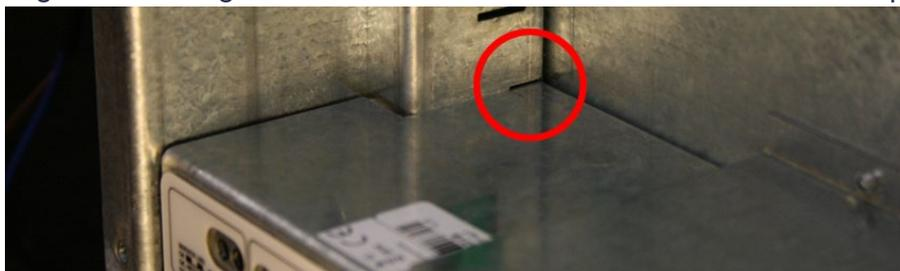
4. Secure the module using the fixing screw on the right. The unit should sit securely with no movement.
