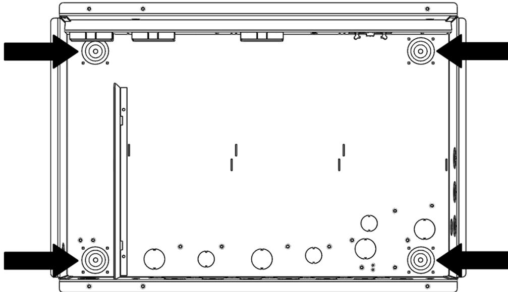
Recess mounting is supported by four mounting holes suitable for M6 (1/4") fasteners, two on either side of the enclosure as shown below.
