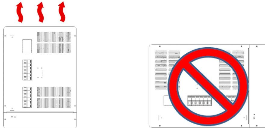
The DMC2 requires an air gap of at least 200mm (8 inches) on all sides of the front cover for adequate ventilation. This gap also ensures that the device is serviceable while still mounted.
