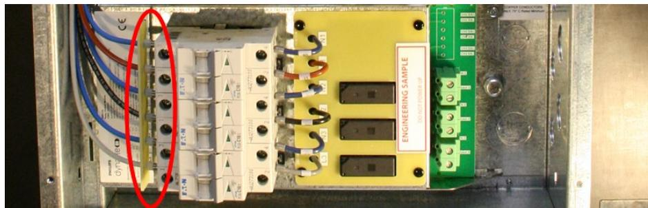
7. Recheck all terminal screws and tighten.
