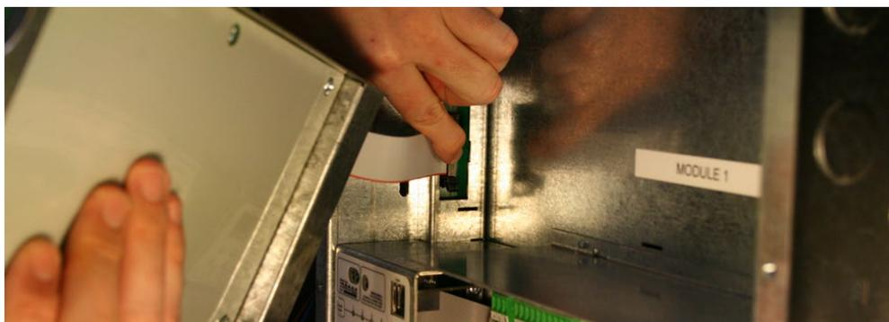
3. Locate the tab and slide the module into position.
