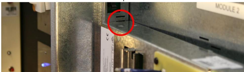
4. Secure the module using the fixing screw on the right side. The unit should sit securely with no physical movement.
